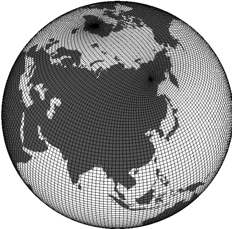
Figure 4: Alternative tripolar model grid with improved grid properties in the Arctic Ocean.
