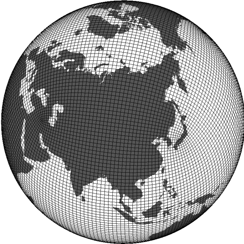
Figure 2: A cubic conformal grid, where a cube is mapped onto a sphere, in this case such that each face has an equal area.
